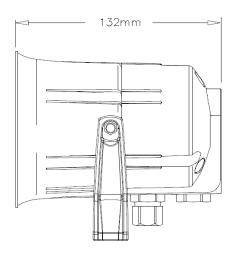
1xM20 cable gland 1xM20 blanking plug cable diameter 6 — 12mm
