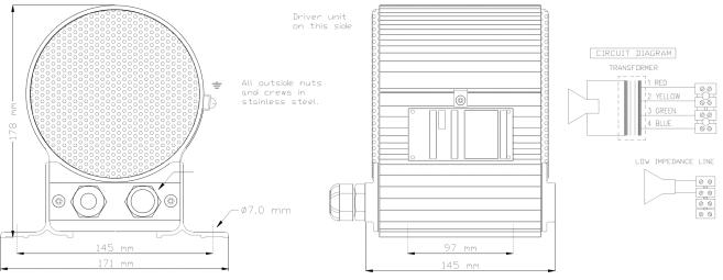
Standard model delivered with two M20 Ex approved plastic blinding plugs
