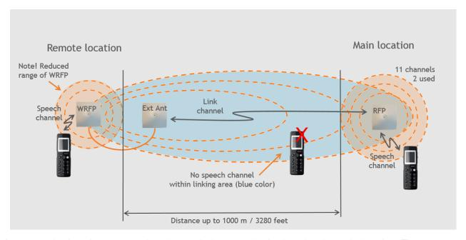
A repeater is placed at a remote location and a base station is placed at the main location. They are too far away to allow the repeater to extend the coverage of the base station. Therefore, an external antenna can be used to establish a connection between the two end points. As the external antenna is a high gain directional antenna, it must point towards the base station you want to link with.
