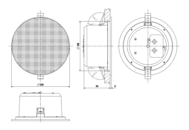
Measurements according to DIN IEC 268-5
