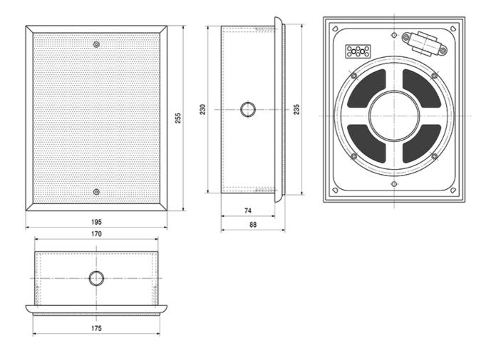
Measurements according to DIN IEC 268-5
