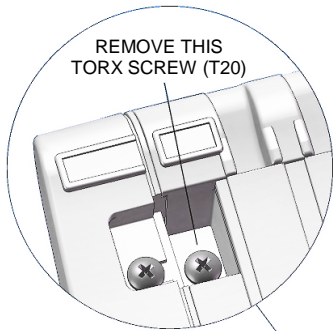
Figure 7 Removing the case bottom half
