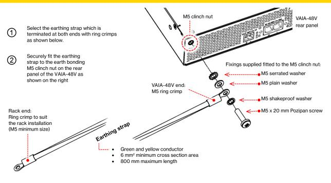
3 Securely connect the earthing strap to the rack at a suitable location using appropriate fixings.
