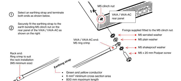
Securely connect the earthing strap to the rack at a suitable location using appropriate fixings.
