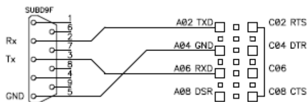
Figure 82. Cable wiring for BusinessPhone
