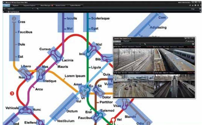
To ensure immediate incident detection, system alarms can notify users of certain events, or if the equipment is malfunctioning. Alarms from all connected security devices and systems are shown in the **interactive map** where alarms from sub-maps are propagated to the primary map.
